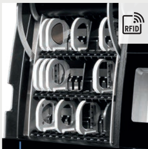
Integrated and RFID-controlled blank tank
